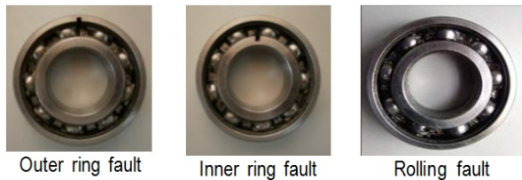
Fig. 7. Fault 6206 ball bearings used in the experiment.
