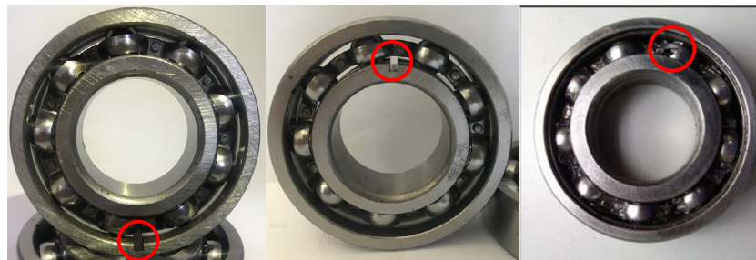
Fig. 20. 6206 ball bearing of outer race fault, inner race fault and ball fault.
