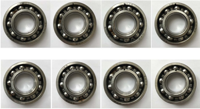
Figure 10. The faulty bearings with localized defects on raceways.
