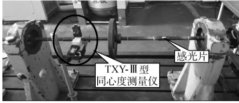
图 13 百分表测量转子弯曲实物图 Fig. 13 Physical map of bended rotor by dial indicator measuring
