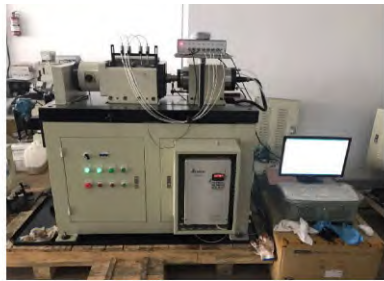
(a) ABLT-1A bearing fatigue strengthening testing machine
