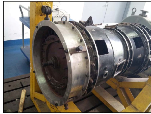
Fig. 7. Thick-walled casing after installation.
