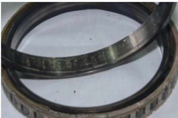
(a) 轴承外环滚道剥落、挤压
