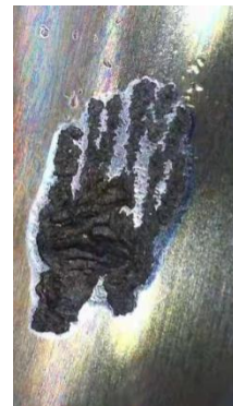
(c) 故障剥落形貌
