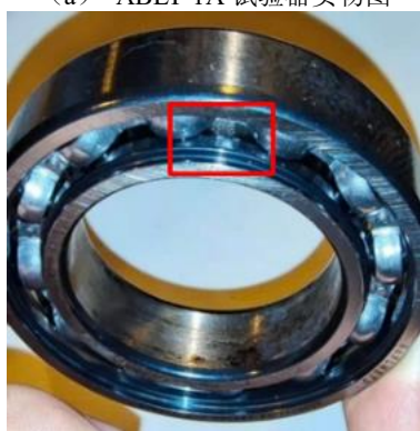
(c) 2 号轴承内圈剥落故障
