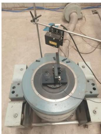
(c) 1 号裂纹叶片一阶弯曲—
