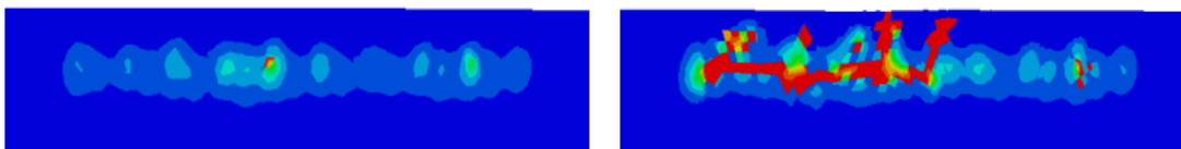
(a) 裂纹萌生, N = 1.786 \times 10^7
