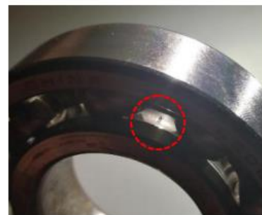
(c) 3号剥落轴承, N=5.57 \times 10^8 1.80 mm
