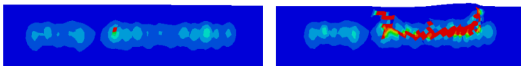
(a) 裂纹萌生, N = 1.773 \times 10^7
