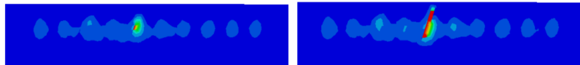
(a) 裂纹萌生, N = 4.155 \times 10^9
